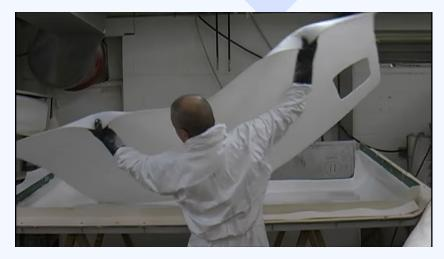
Below showing the further layer of matting being applied onto the Nidaplast:
