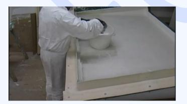
After resin is applied you can then consolidate with a consolidating/paddle roller. This technique is used to ensure trapped air is released and the matt is fully impregnated with resin.
