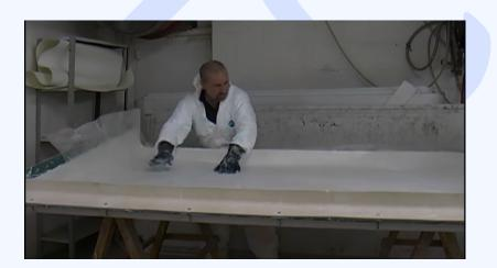
Only a very light coat of resin is needed for the tissue application, surface tissue <u>https://www.ecfibreglasssupplies.co.uk/surface-tissue</u> will improve the final finish to the chopped strand.
