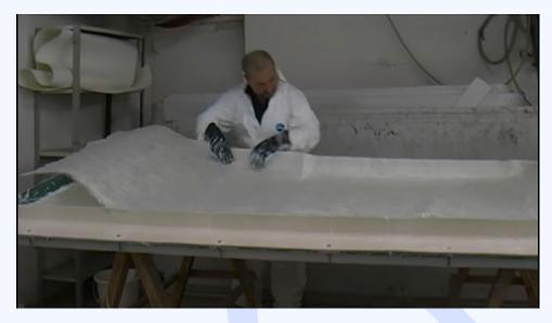
More catalysed resin is added once the matting is in place. Be careful not to oversaturate. Resin to Glass ratio should be approx. 2.5kg resin to 1kg matt.
